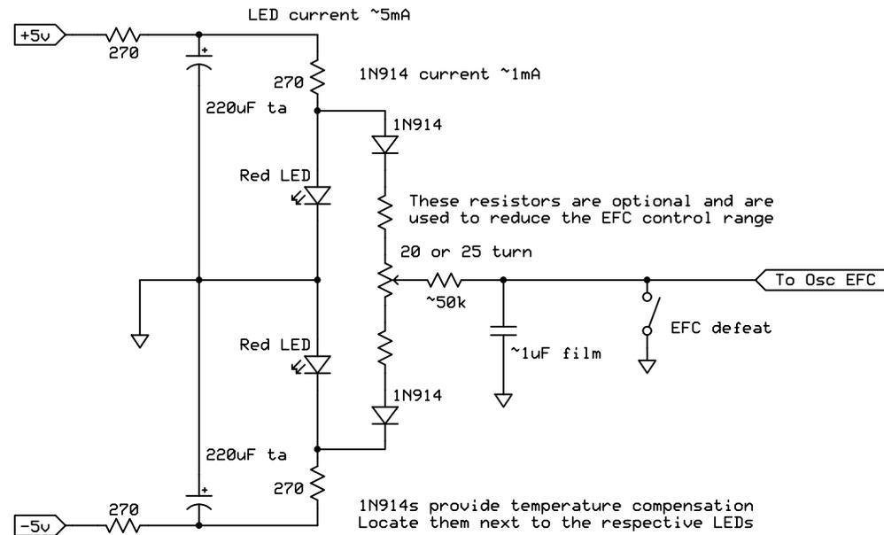
Divider string voltage (between 1N914s) is ~ +/- 1.2v
