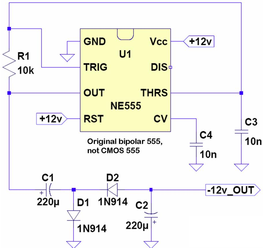
With C3 = 100n, oscillator runs at ~700Hz
